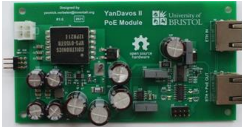
Fig. 6. Power over Ethernet (PoE) injector designed for YanDavos II, with the 48 V step-up converter with isolation transformer to the left, and the Ethernet controller to the right.
