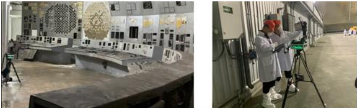
Fig. 4. YanDavos II static deployments on a tripod, as seen inside the Unit 4 Control Room (left) and while imaging the western wall of the Shelter inside the NSC (right).
