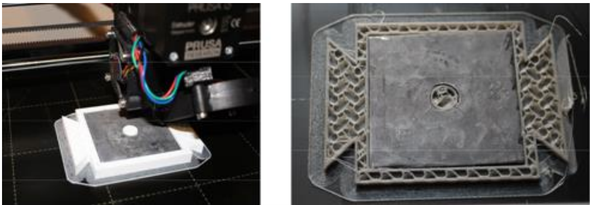
Fig. 7. 3D printing lead-containing composite materials for shielding of sensitive components in YanDavos II
