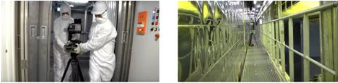
Fig. 8. YanDavos II being transported inside the NSC by ChNPP staff (left) and as seen during a scan from a suspended walkway (right).
