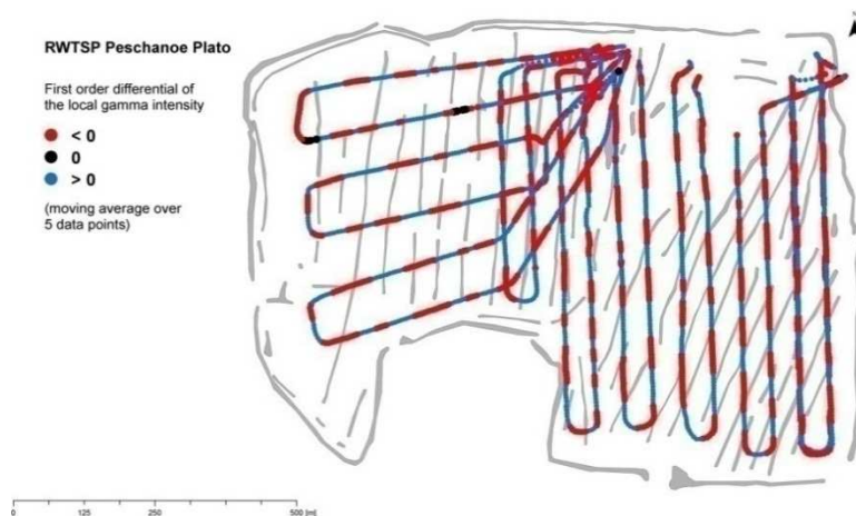
Figure 10. Calculation of the first differential of the local gamma intensity to identify burials at RWTSP Peschanoe Plato [5,7]
