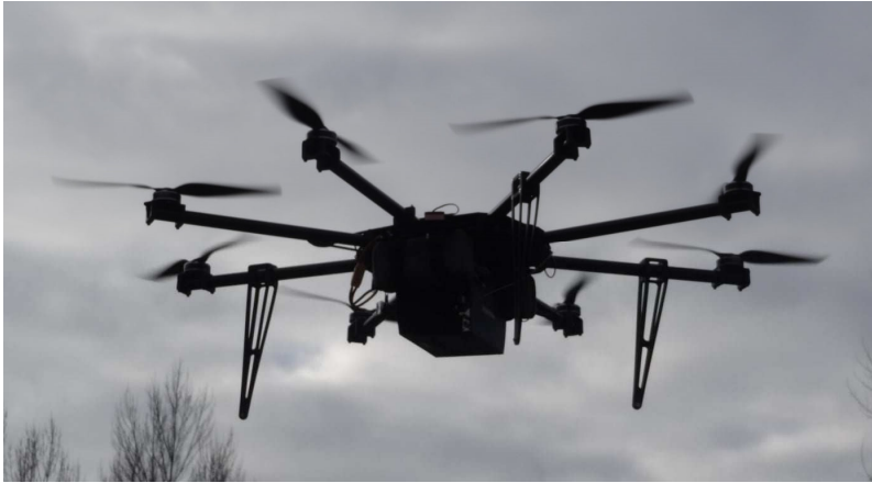
Figure 11. YellowScan Mapper (black box at the bottom) mounted on the Octocopter. Results of new gammaspectrometric surveys shown as flight traces on the existing contamination maps
