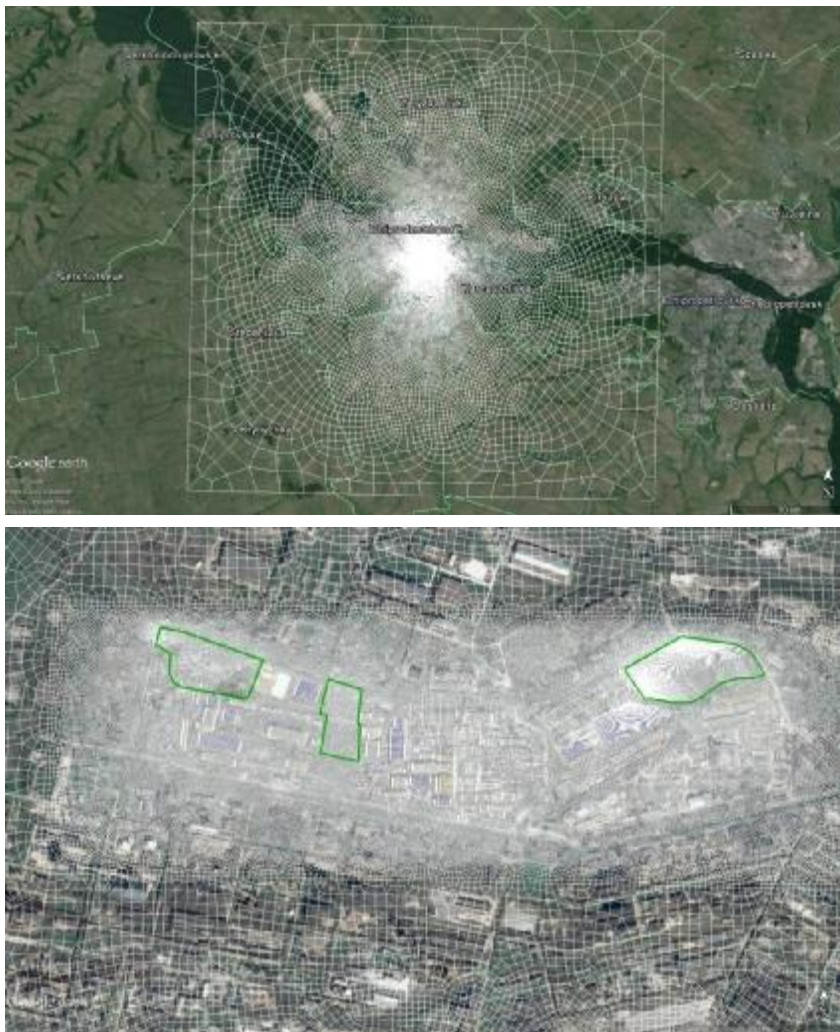
Figure 4 – Computational domain and unstructured grid for Open Foam application on a range of scales (from local to mesoscale) at the territory of PChP. Upper – full extent of the domain, covering PChP industrial area and living zone of nerby Dniprodzerjinsk city; bottom – grid at the industrial site of former PChP (resolution down to 5 m)
