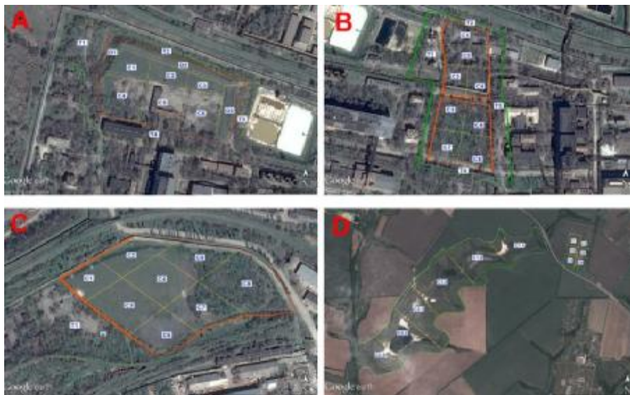
Figure 1 – Dividing of tailings ‘Zapadnoe’ (A), ‘Central Yarr’ (B) and ‘Yugo-Vostochnoe’ (C), Sukhachivske and Base C (D) onto sectors
